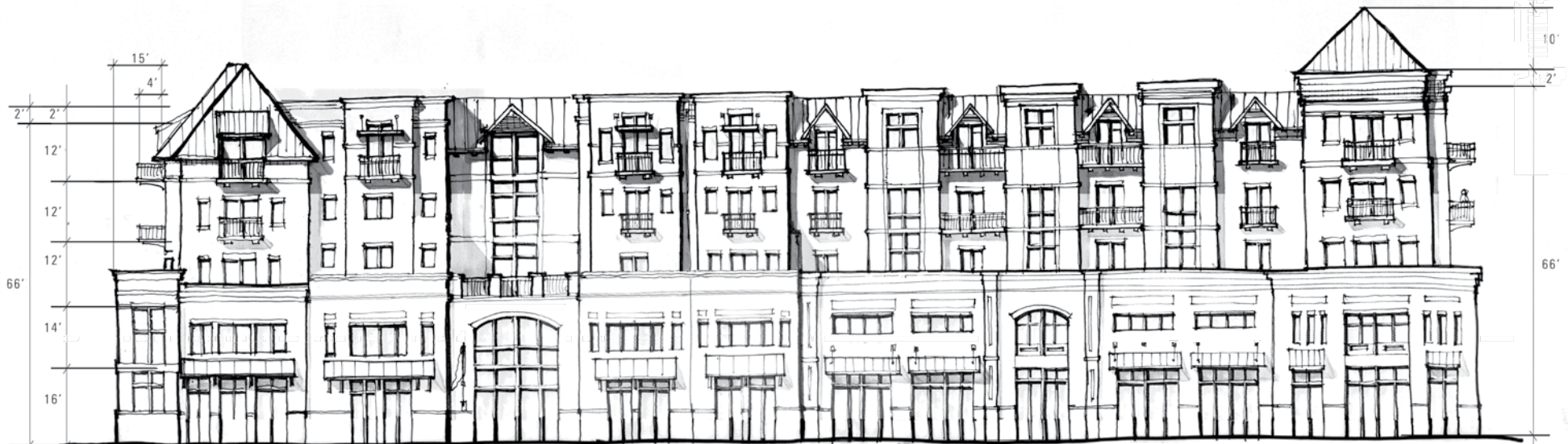
CONCEPTUAL ILLUSTRATION OF STEP BACK FLAT ROOF WITH LIMITED AREA OF PITCHED ROOF
